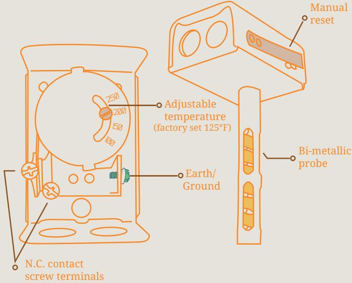
The helix bi-metal element is mounted into a 0.750" inch O.D. hole on the air duct. The bimetallic probe monitors the temperature in the duct based on the field adjust-able setting chosen, or the fixed preset temperature. If a severe change in temperature is detected, the probe expands and actuates the switch. In addition, the firestat can activate an alarm or a set of louvers. The firestat is required to be manually reset acknowledging there was a change in temperature.
